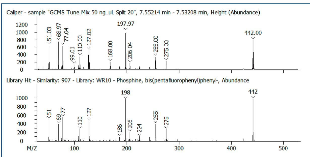
**Figure 3. The Caliper (raw) mass spectrum at the apex of the DFTPP chromatographic peak with a one point background subtraction, and the corresponding library match spectrum for DFTPP, show that the Pegasus BT routinely passes DFTPP tuning.**
