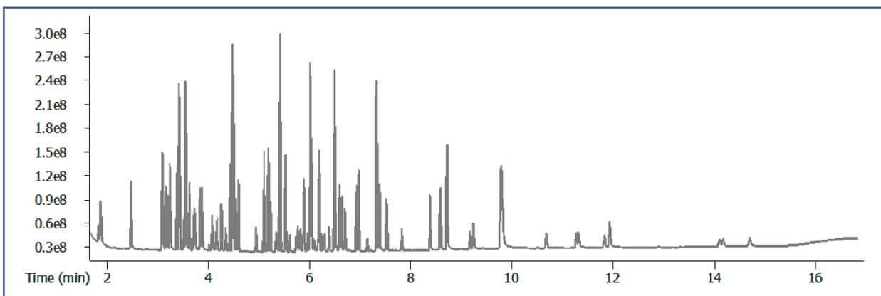
**Figure 2. Total ion chromatogram (TIC) of a 5 ppm standard containing 90 components.**
