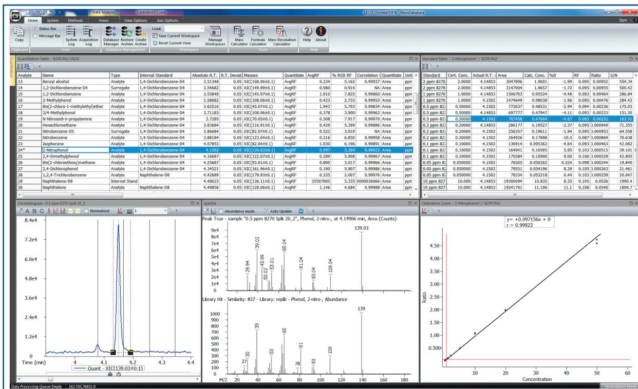
Figure 5. Quantitation using ChromaTOF 5.0 to evaluate calibration data for 8270 compounds. The highlighted compound is 2-Nitrophenol.
