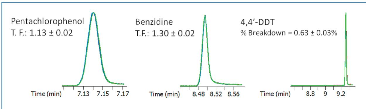
Figure 4. Check of the GC column performance and injection port inertness.
