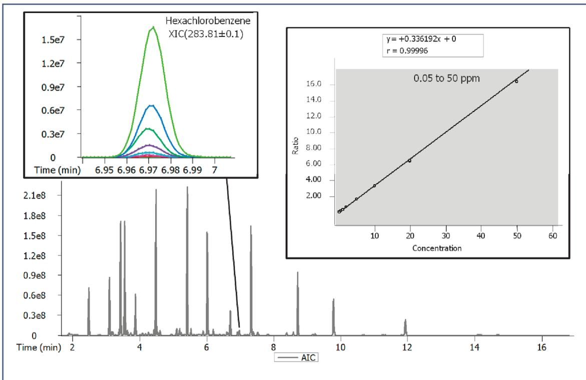
Figure 1. Extracted ion chromatogram (XIC) of the quant mass for hexachlorobenzene (HCB) from 0.05 to 50 ppm and its corresponding calibration curve, with the Analytical Ion Chromatogram (AIC) of a 1 ppm standard split 20:1 indicating where HCB elutes in the chromatogram.
